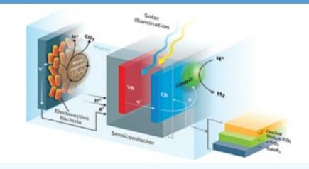
**CONTEXT** – A self-sustaining microbial photoelectrosynthesis system is paired with photoelectrochemical water reduction for energy efficient  $H_2$  generation. In other words, bacteria treating wastewater, generates electrons that are used to generate  $H_2$  from water.
