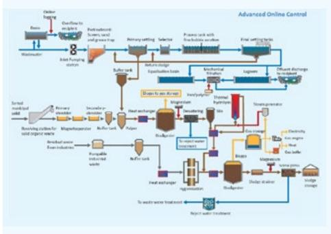
**CONTEXT** – Billund BioRefinery is a publicly owned company providing services in water supply and waste management to the municipality of Billund. It was established in 1997 as a WWTP co-digesting industrial and municipal bio-waste with wastewater sludge. The plant was upgraded to a Bio-Refinery in 2016 to increase biogas production, minimise energy consumption, enhance process control and improve effluent quality.
