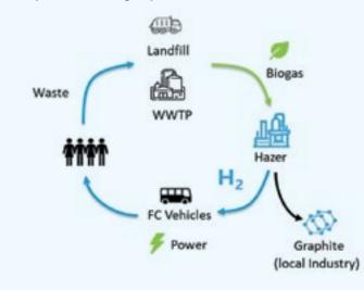
**CONTEXT** – The Hazer process will be constructed to convert bio-methane generated at Woodman Point WWTP in Munster, WA, to hydrogen and graphite using an iron ore catalyst and creating an alternative pathway to the traditional approaches of steam methane reforming and electrolysis.
